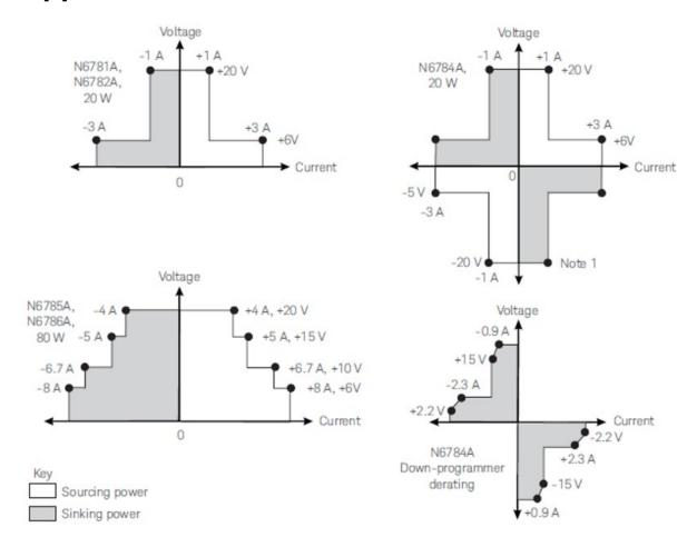
Note 1. When sinking power, the N6784A model can operate at the maximum rated output power for only a limited amount of time. The unit monitors the temperature of the internal power devices and latches the output off if the output power has exceeded its safe limits. A protect clear is required to resume normal operation. The condition is annunciated by the OT status bit. Refer to the down programmer derating figure for the values of the safe limit boundaries.
