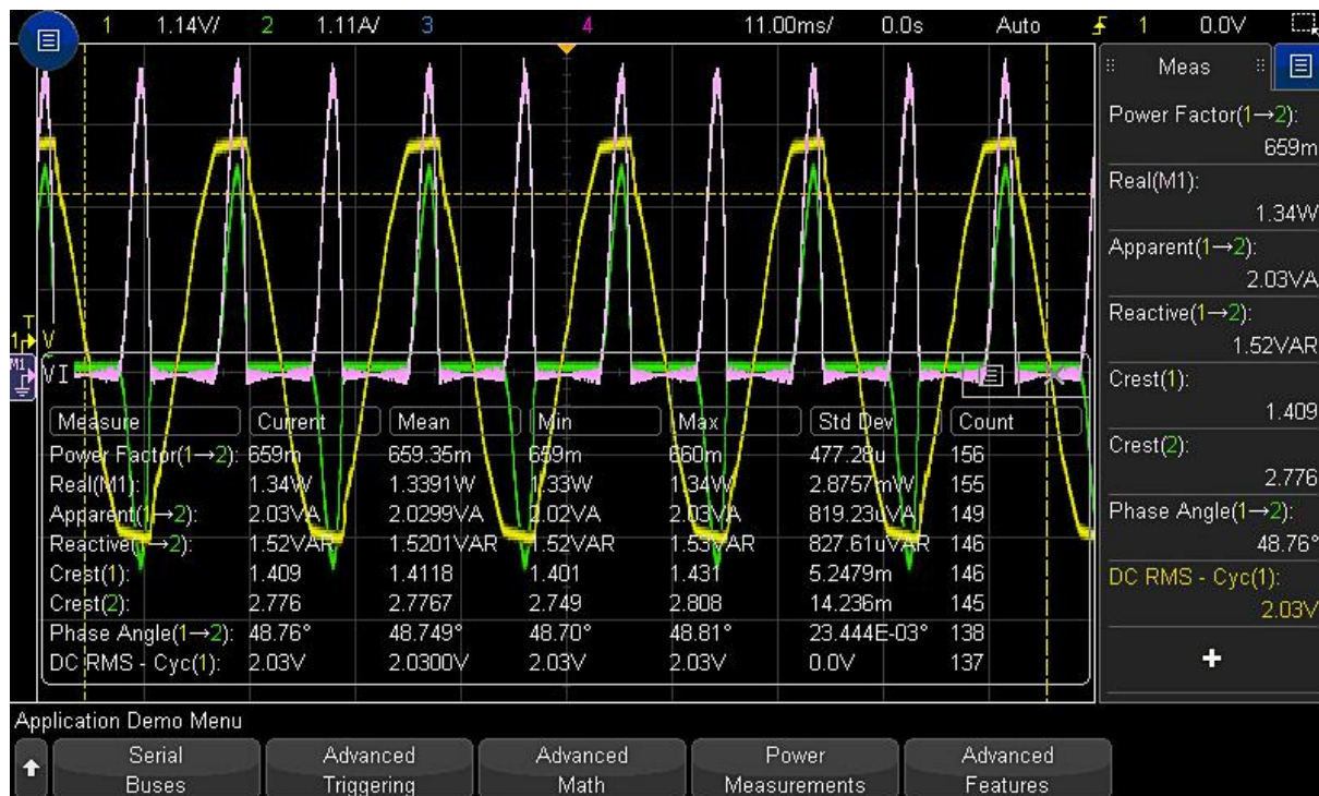
Figure 33. Integrated power measurements make quick work of analyzing power producing and power consuming devices.
